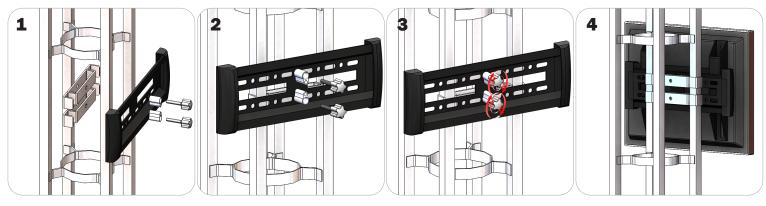
Locate all components needed to assemble the monitor mount with the Vertical Orbital Truss method. You will need (1) monitor bracket, (2) OR-TVA-PBKT-1 brackets, (2) OR-KNOB-2, and (2) spacers. Determine your desired monitor location.
