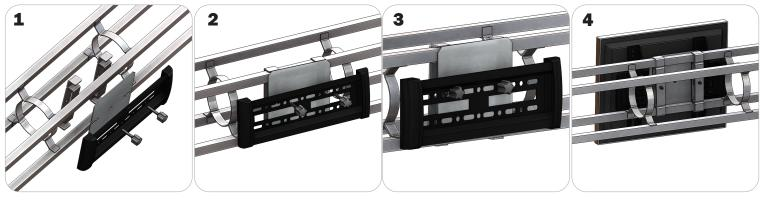
Locate all components needed to assemble the monitor mount with the Horizontal Orbital Truss method.
